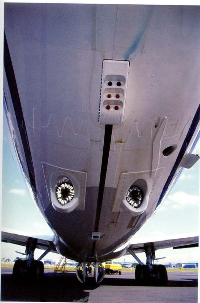
ABOVE: A close look at the underside of Omega's 707AR tanker/transport reveals its special features, namely the twin refuelling baskets in the retracted position, refuelling readiness lights and, further forward, the twin-lens video camera that monitors the refuelling process. Author
