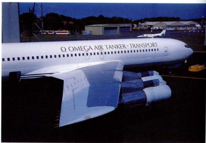
BELOW: The 707-320B (as seen here) featured several improvements over the standard -320, mainly to the wing. These included curved, low-drag wingtips, full-span leading-edge flaps and larger trailing-edge flaps. Author
