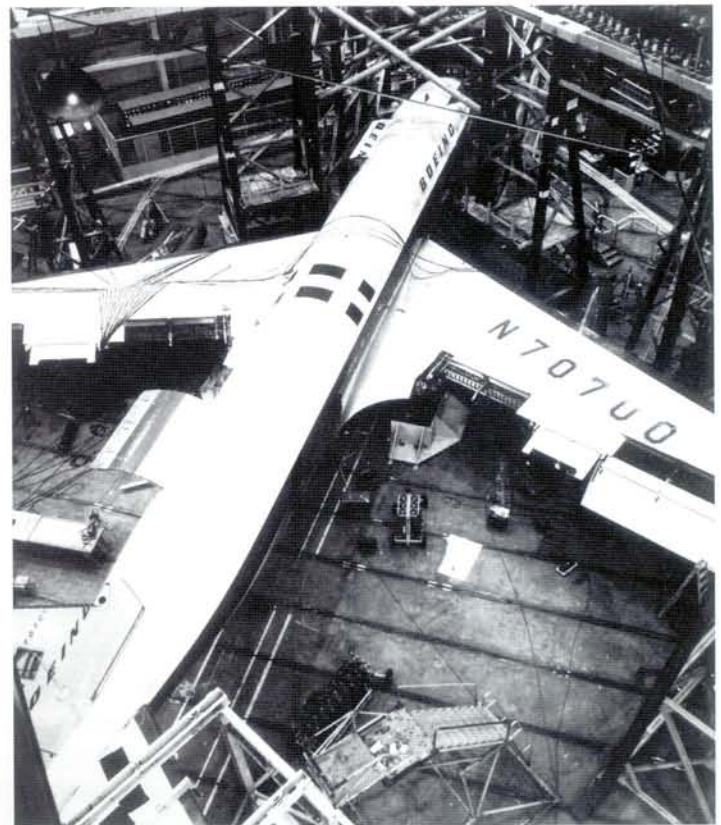
BELOW: As well as static rig tests as seen here, a full water tank test was made of a 707 fuselage. Boeing's engineers were avoiding the mistakes of the Comet, which was not as rigorously tested, with disastrous consequences. Sabena via Aeroplane
