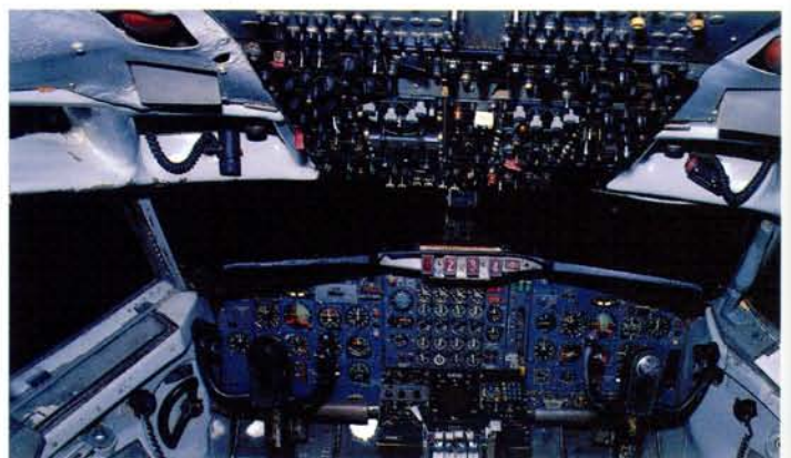
BELOW: Boeing 720 cockpits were basically the same as those on 707s, and airlines with both types in their fleets cross-qualified their crews to fly either as required. Seen at Luton in March 1981, this was the cockpit of Monarch Airlines' G-AZNX, a former TWA and Northwest Orient aircraft. It served with Monarch from 1972 to 1983 when it was sold to the Boeing Military Airplane Company and stripped for parts at Davis-Monthan AFB, Arizona. Austin J. Brown/The Aviation Picture Library
