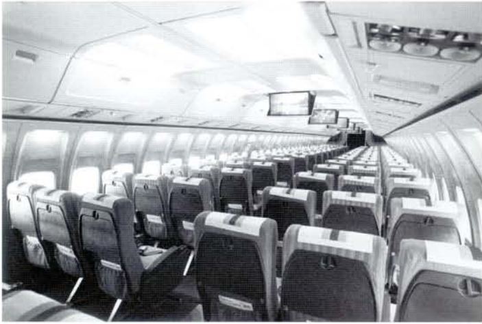
ABOVE: Many airlines revamped their 707s in the early 1970s. New lighting, overhead bins and service unit panels, and such things as in-flight movies, were an attempt to compete with airlines with new equipment such as 747s. Demonstrating the 'wide-body look' here is a 1971 American Airlines 707-300 'LuxuryJet' cabin. American Airlines via Author
