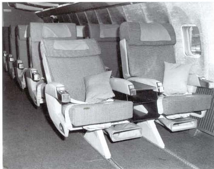
ABOVE: The 707's seat tracks could accommodate two- or three-seat units, allowing for four, five or six abreast seating arrangements. This is the first class seating in a BOAC 707-400. Moveable divider panels allowed easy reconfiguration between classes. The overhead passenger service units or 'pods' were also moveable to suit different seat arrangements. BOAC via the Aviation Picture Library
