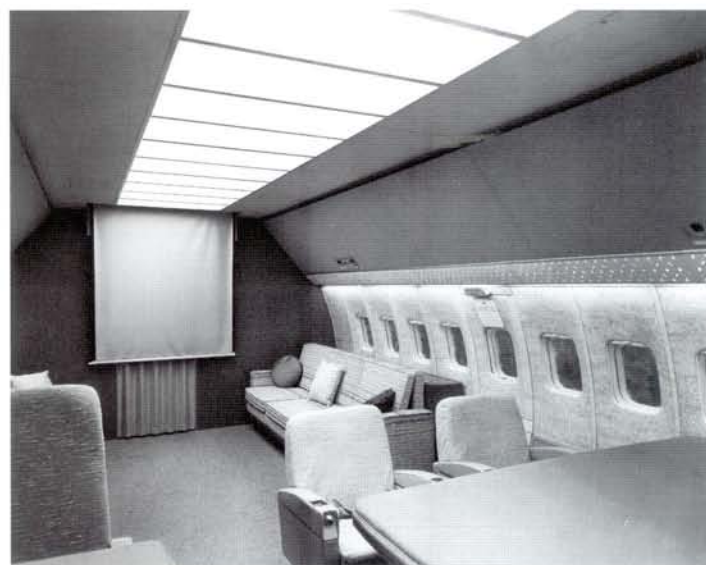
BELOW: This is the conference room of one of the USAF's first three VC-137As, located at the centre section of the aircraft. The projection screen was for in-flight briefings and the sofas on each side converted into bunks. Boeing via Aeroplane
