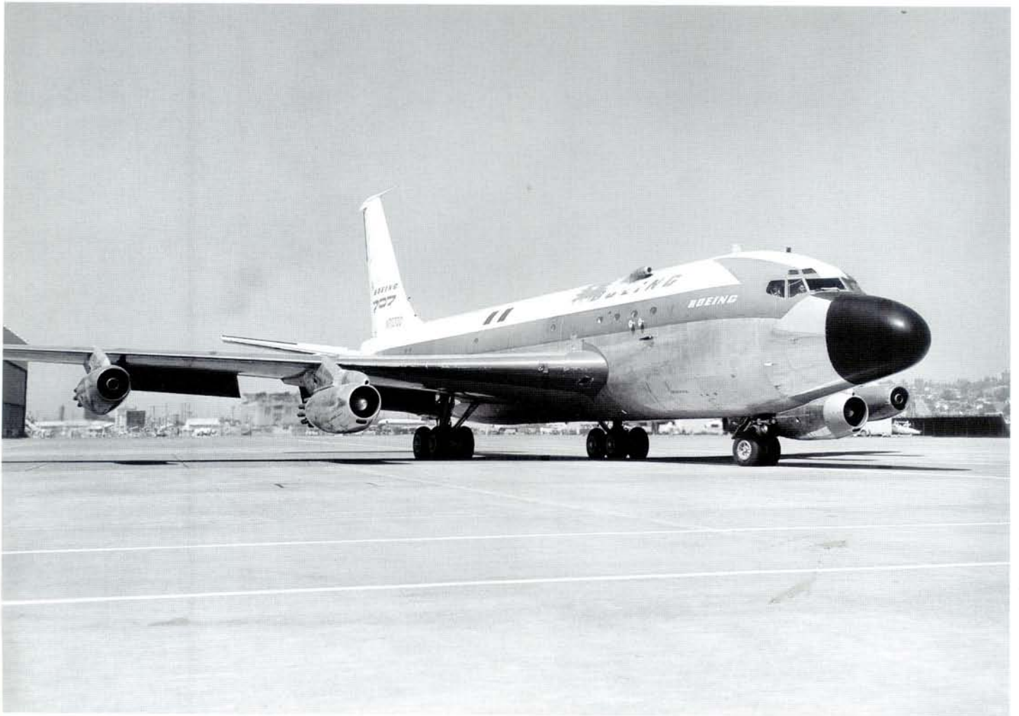
ABOVE: Another modification to the Dash 80 saw the addition of a large radome for the Bendix AN/AMQ-15 weather reconnaissance radar. Extra equipment collected high-altitude atmospheric data and monitored drop and rocket sonde weather probes. This nose appears to have come and gone within 1959. Boeing via Aeroplane
