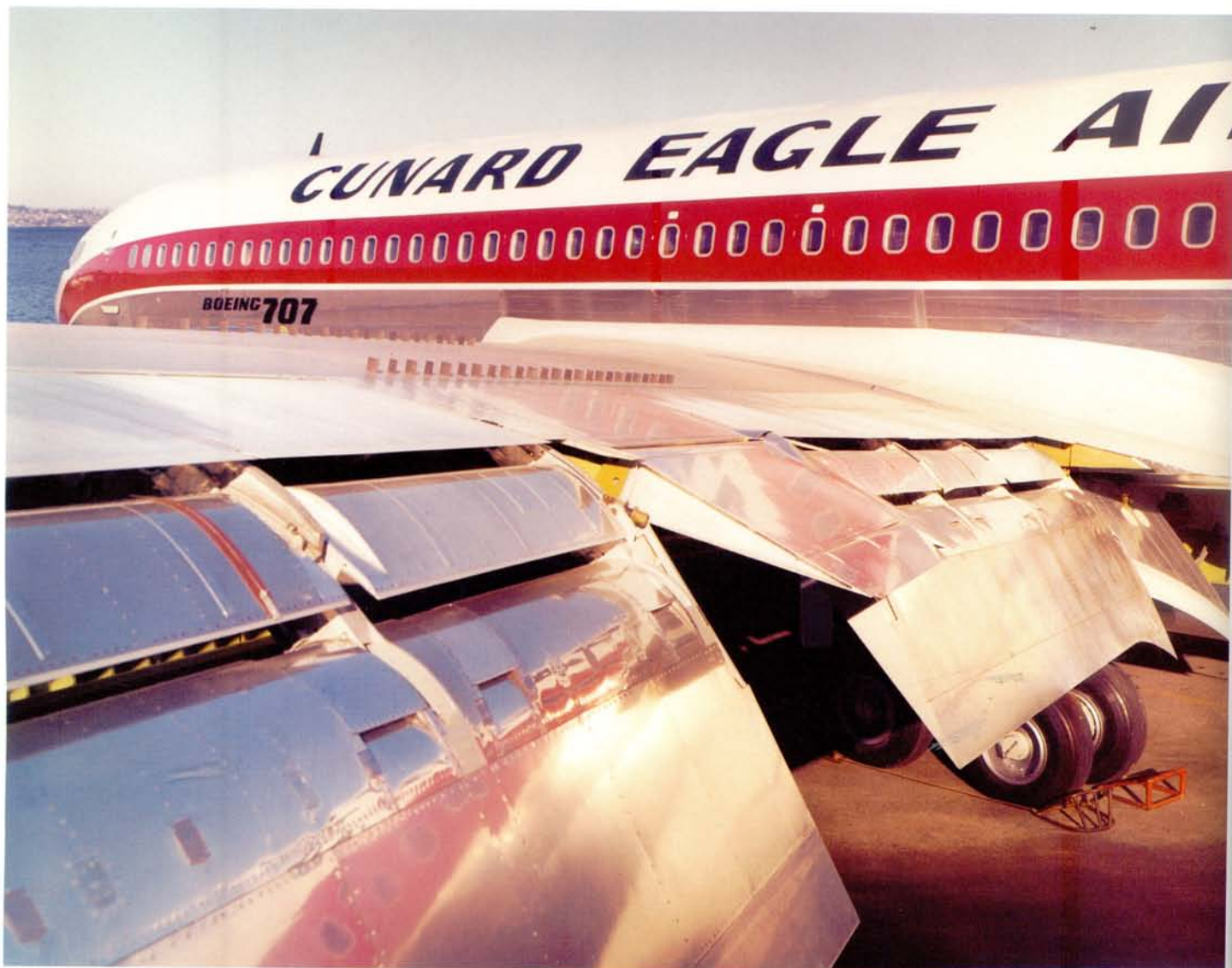
ABOVE: Some of the complexity of the 707's control surfaces can be seen here, including the triple-slotted flaps and the inboard aileron. Vortex generators placed ahead of the inboard aileron cured a tendency for the wing to shake in high-speed cruise. Boeing via the Aviation Picture Library
