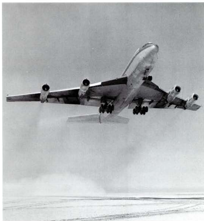
BELOW AND RIGHT: As part of tests for the very large aircraft (later C-5) programme, a double-wheel undercarriage was installed on the Dash 80 and many take-offs and landings were made on the Harper Dry Lake, California in 1959. The temporary landing gear was not retractable. Boeing via the Aviation Picture Library
