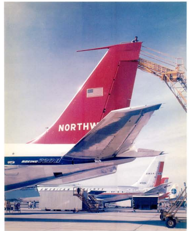
BELOW: The tail surfaces of this Northwest Orient 720B shows the distinctive high frequency (HF) antenna on the fin which was not specified by all 720 operators, but was later refitted to many aircraft. The shallow ventral fin used on the 720s is also well shown. Boeing via the Aviation Picture Library
