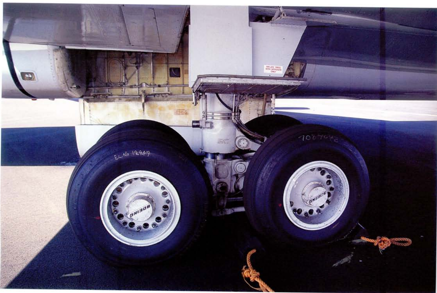
ABOVE: The starboard main landing gear unit of a 707-321B. The -300C had a stronger undercarriage to allow for greater landing weights and different brakes, Goodyear as opposed to Goodrich multiple-disc units. Author
