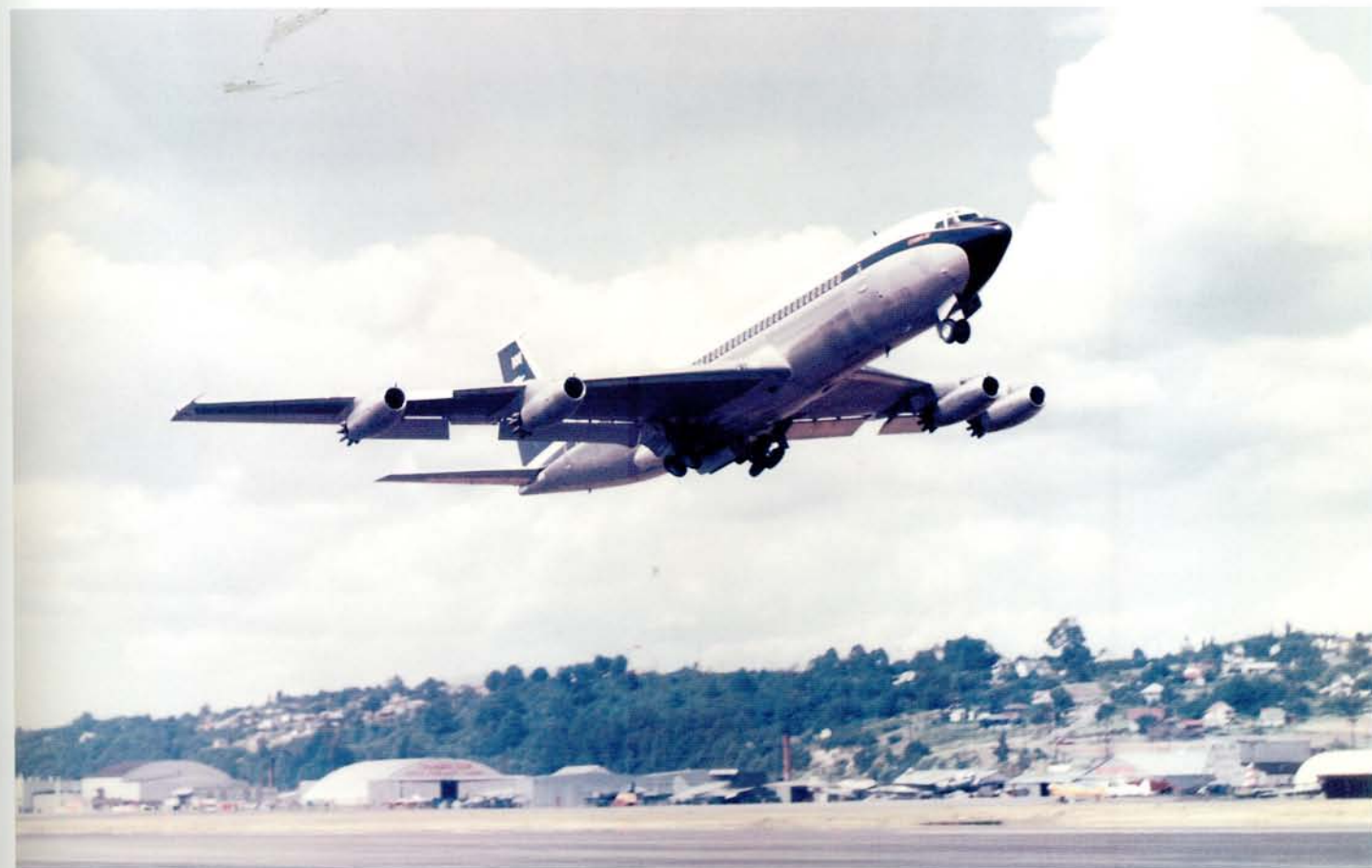
BELOW: A BOAC 707-436 lifts off from Renton under the power of four Rolls-Royce Conways. The certification programme for BOAC's jets was long and complex. First flown in May 1959, FAA certification took until February 1960 and the British nod was another two months in coming. A taller tail and a new underfin would be needed before the -436s were ready for delivery. John Stroud Collection/The Aviation Picture Library
