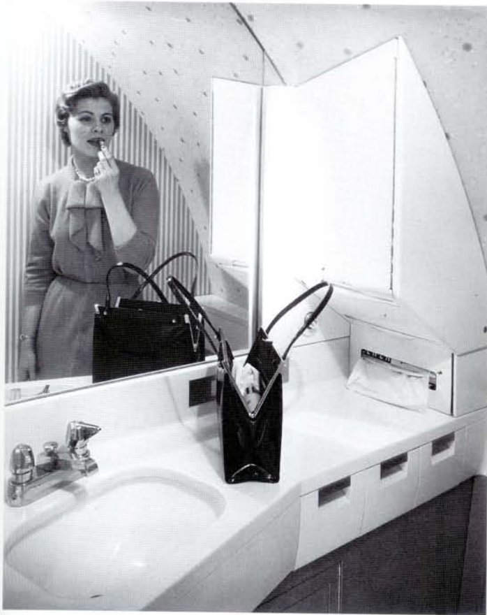
ABOVE: The lavatories of the 707-100 were designed to 'duplicate the effect of a small powder room in a family home'. Note the curve of the wall – the aft lavatories were in the tapering part of the rear fuselage. This is actually a view of the $500,000 cabin mock-up constructed in a New York warehouse by Walter Dorwin Teague and Associates. Boeing via Aeroplane
