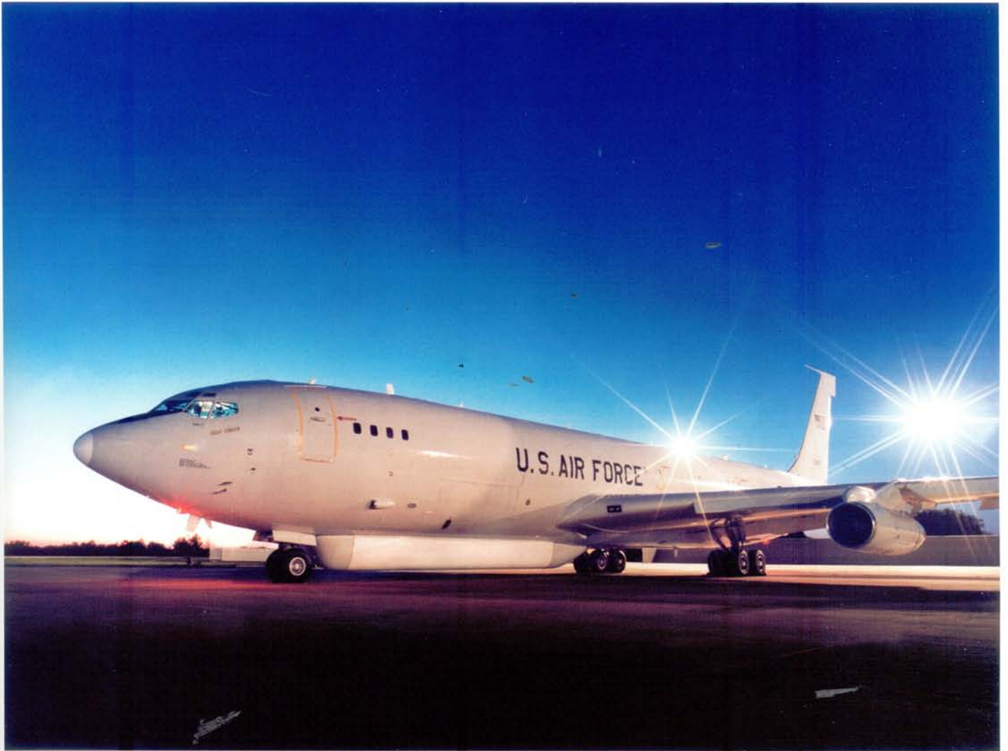
ABOVE: The Northrop Grumman Joint Surveillance Attack Radar System (Joint STARS or J-Stars) is the official name for an ex-airline Boeing 707-300 converted to a sophisticated airborne targeting and battle management platform. Officially in service from late 1997, the J-stars was trialled successfully in the 1991 Gulf War. Northrop Grumman via the Aviation Picture Library
