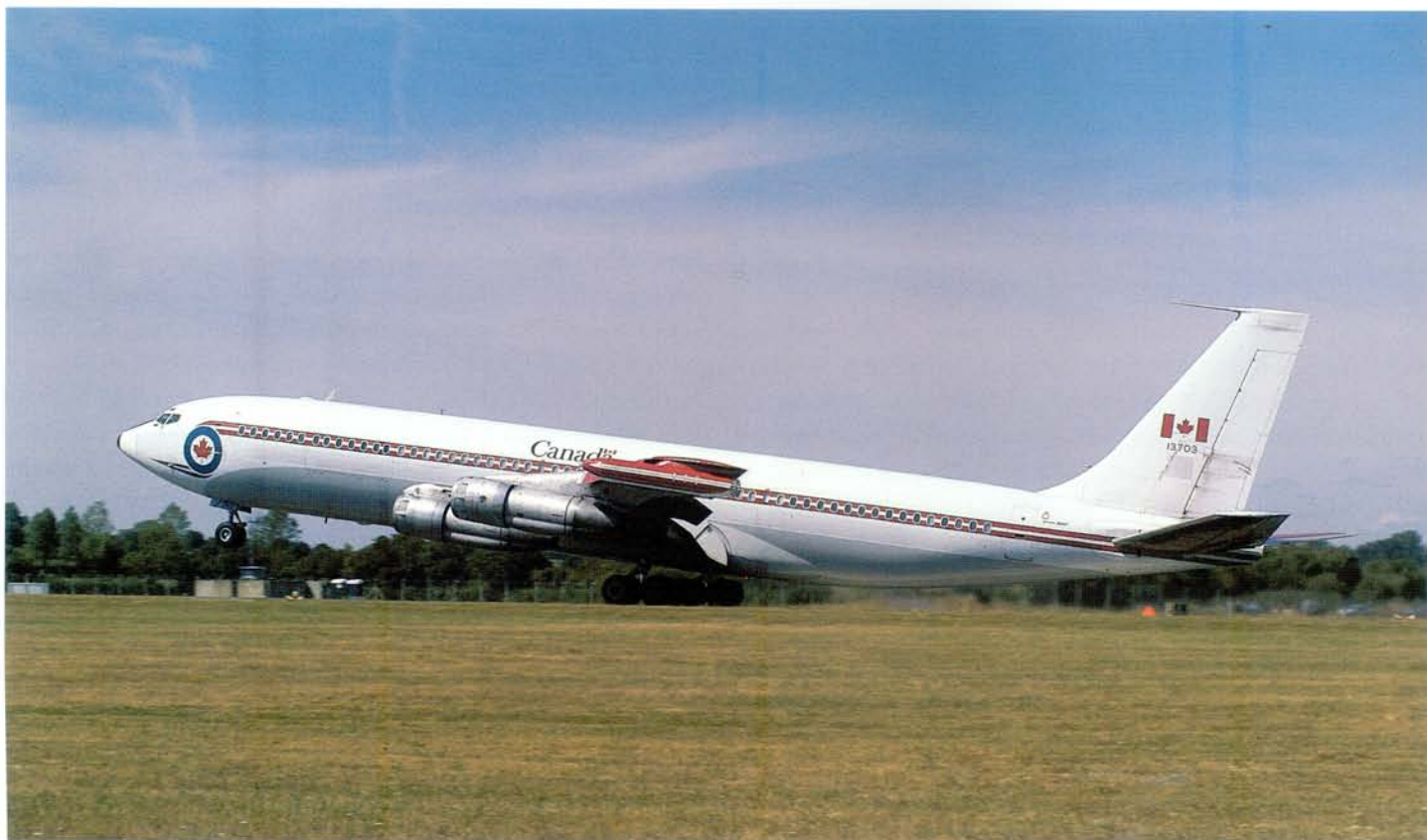
ABOVE: Canada operated a fleet of five Boeing 707s or CC-137s in the tanker and transport role. They were replaced as transports by Airbus A310s (or CC-150 Polaris) twinjets in 1997, but it was not until late 2001 that a decision was made to equip two of the five Airbuses as aerial refuellers. Austin J. Brown/ the Aviation Picture Library
