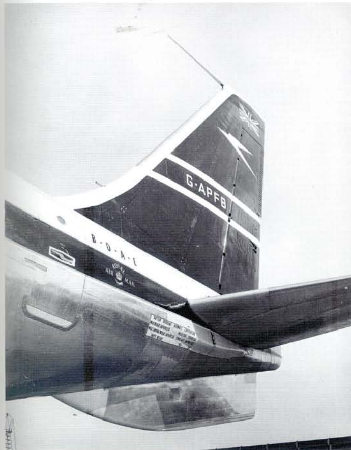
BELOW: The so-called ARB fin on 737-436 G-APFB. When the marginal stability characteristics of the 707 in some modes was realised, Tex Johnston, backed up by the aerodynamicists, recommended a taller fin, a boosted rudder and the ventral fin seen here. Bill Allen and Boeing's board accepted his findings, as did the British. Johnston answered BOAC's question, 'Who pays for it?' with 'Boeing' – an answer that reassured the customers and ensured the success of the 707, but which delayed profitability even further. Boeing via the Aviation Picture Library
