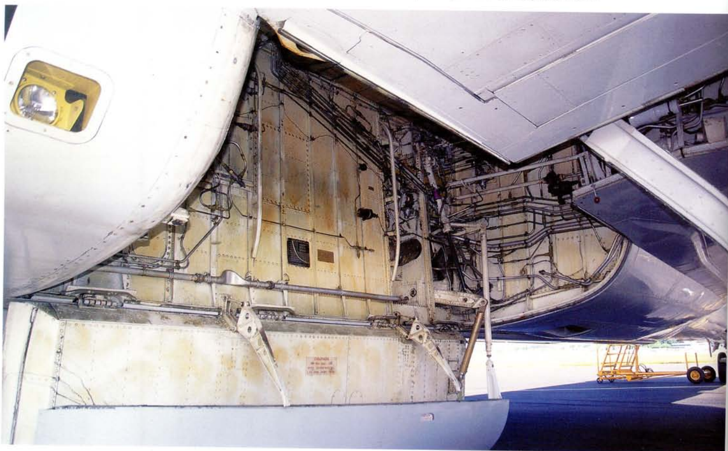
BELOW: The mainwheel well bays of the 707-300 were usually enclosed by doors except when retracting or extending, but could be opened on the ground for access to the hydraulic panel and other equipment. Author
