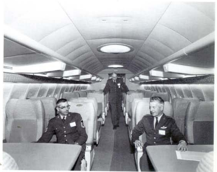
ABOVE: The aft cabin of the VC-137A contained fourteen sets of double seats and four tables. The forward cabin contained a communications centre with a high-frequency communications set and radio teletype machine as well as the usual galley and toilets and an eight-person seating area. Boeing via Aeroplane
