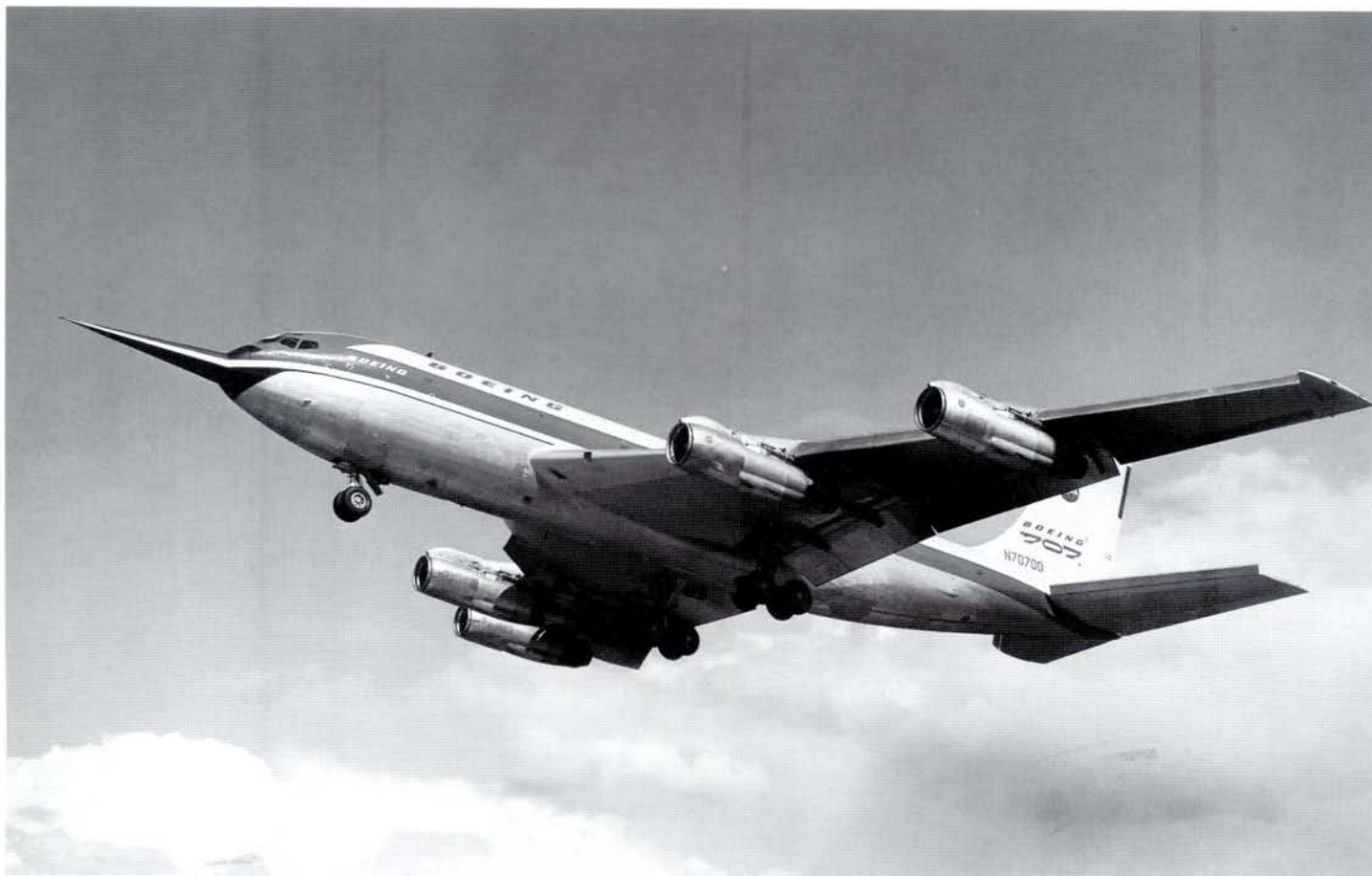
ABOVE: As part of 1963 tests into supersonic and very large transports, the Dash 80 mounted a long instrumented nose probe. At this time the wings were modified with a full set of blown leading-edge flaps and a tailplane with an inverted leading edge. Boeing via the Aviation Picture Library
