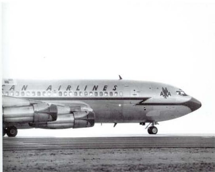
ABOVE: The forward fuselage and engines of an American Airlines 720B are seen at the end of one of Edwards AFB's long runways during testing of the JT3D engine installation. Notice the test equipment visible in the cabin and the centre of gravity marking on the fuselage top. Boeing via the Aviation Picture Library
