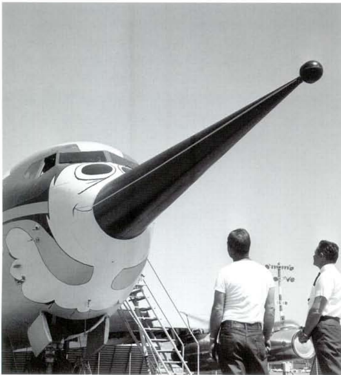
ABOVE: During testing associated with Boeing's proposed Supersonic Transport (SST) in 1975, this 'Pinocchio' nose probe was fitted to the Dash 80. Sensors in the probe fed to a computer in the cockpit that allowed the aircraft's control responses to simulate those of a supersonic airliner or a very heavy transport aircraft. Boeing via Author
