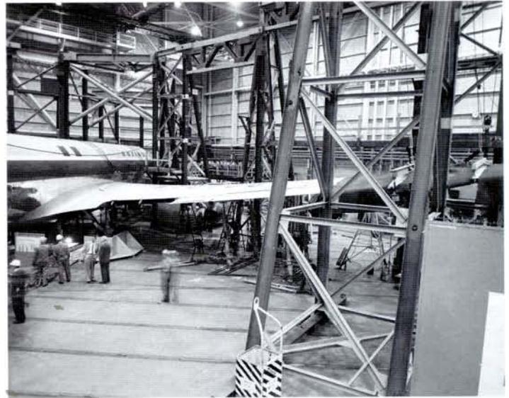
ABOVE: The thin wing of the 707 was designed to flex like that of the B-47, something that airline passengers took a long time to get used to. Structural testing of the Dash 80 saw the wing flexed up to 33 per cent of its design load (failure point) with a deflection of 49 in (124 cm). Aeroplane
