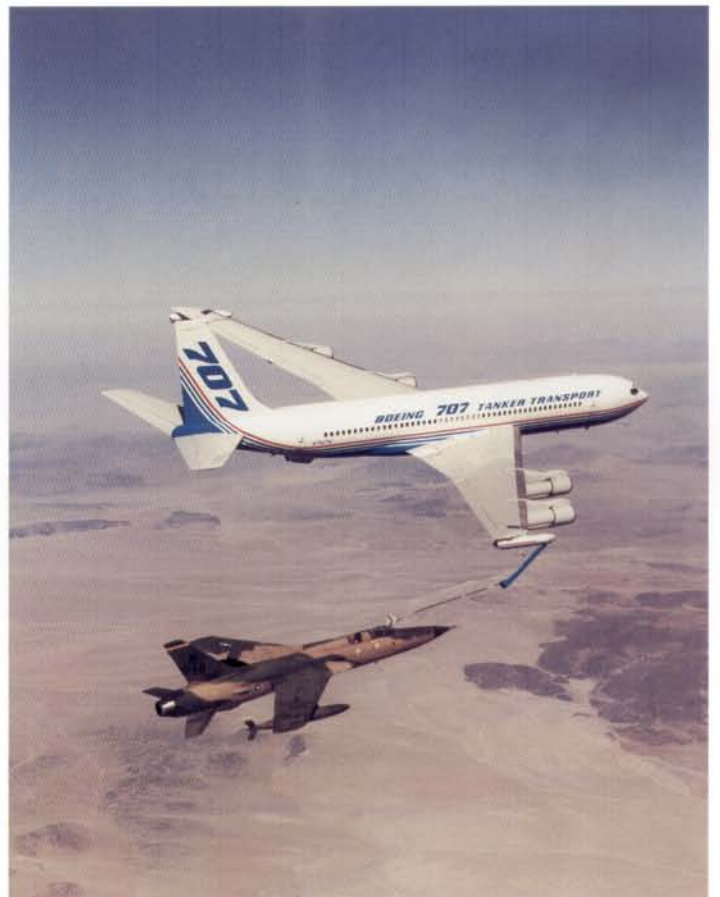
RIGHT: Boeing converted an ex-TWA 707-331C to tanker-transport (also called KC-707 or KC-137E) configuration in late 1982. Like the -3J9Cs built for Iran, the modification involved wingtip pods with a hinged guide chute that lowered the refuelling drogue out of the disturbed airflow. This proved more successful than some third-party conversions using Flight Refuelling Ltd pods, and it was not until 1989 that the aircraft was sold – to Spain as T.17-2. It is seen here conducting trials with an F-105G Thunderchief. Author's Collection
