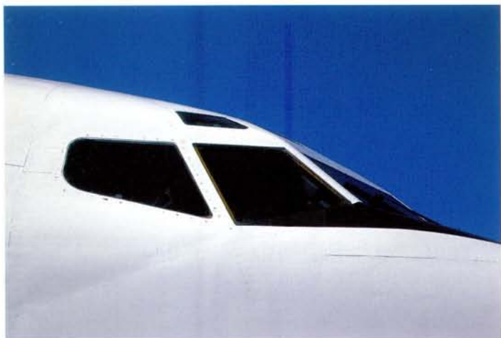
ABOVE: The cockpit window arrangement, nose profile and cabin diameter of the 707 were left basically unchanged throughout production and were adopted for the many 727s and 737s to follow, right up to the New Generation 737s in service today. Author
