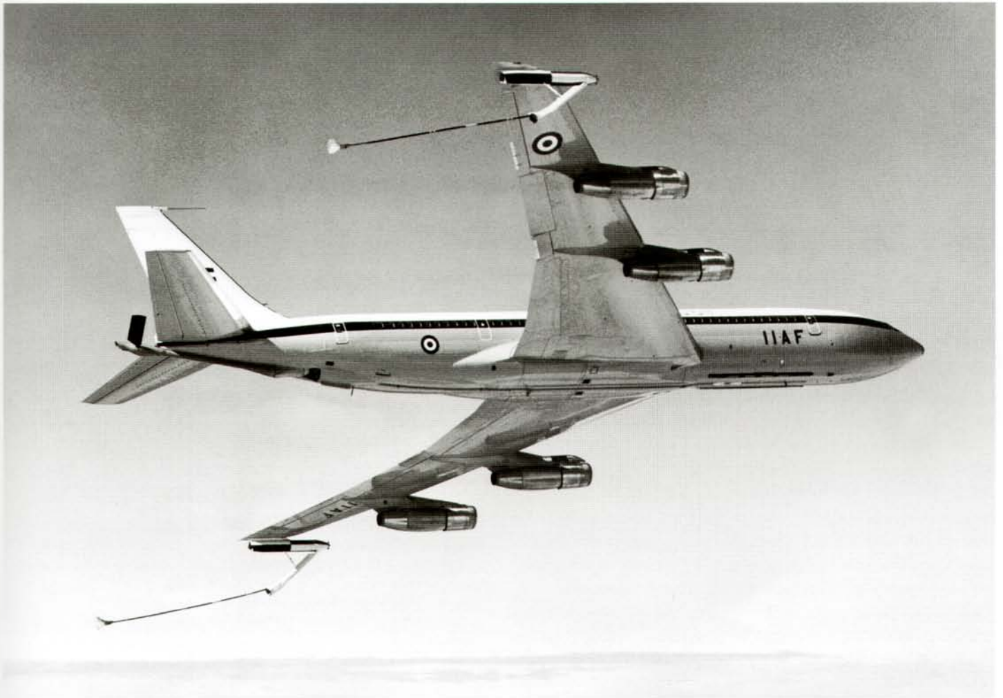
ABOVE: The Iranian (then Imperial, now Islamic Republic) Air Force has been a big 707 user. Their purpose-built -3J9Cs were equipped with both boom and hose refuelling systems. Despite revolution, war and sanctions, most are still believed to be in service at Tehran-Mehrabad Airport. Beech via Aeroplane
