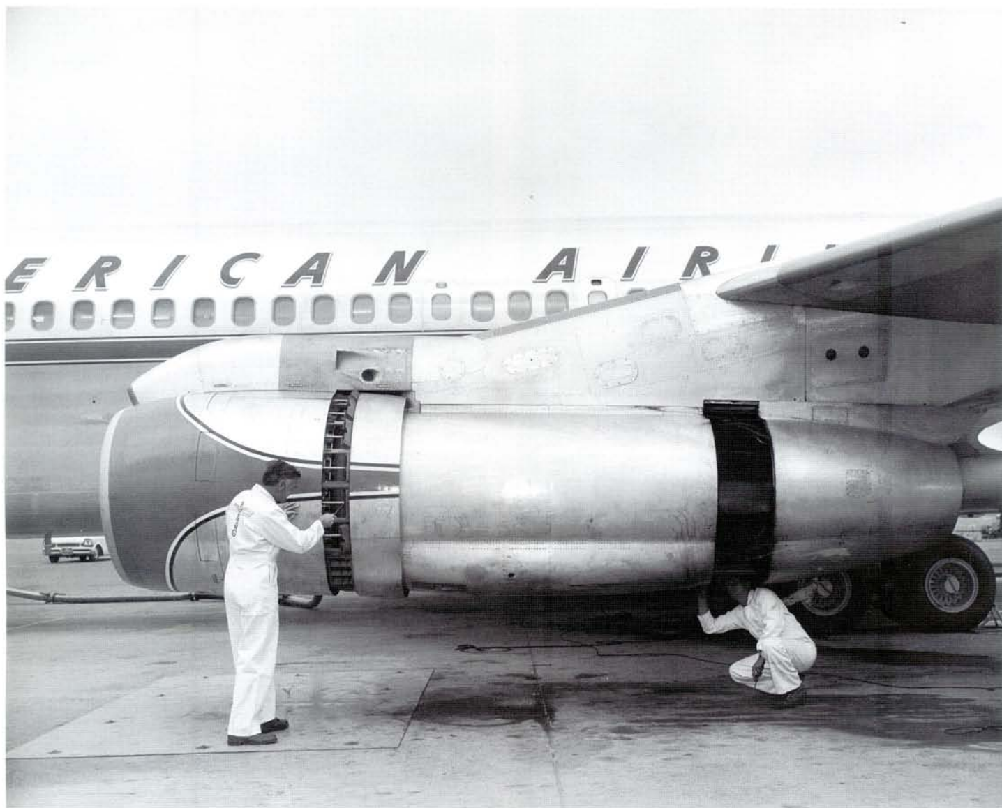
ABOVE: By 1960 707-100s were returning to the factory for conversion to turbofan power. At the same time the opportunity was taken to fit the wing and tail modifications and the whole process took three to five weeks. The JT3C itself was convertible to a JT3D by adding a front fan and a fourth-stage turbine. Accessories were repositioned below the engine for better accessibility. Author's Collection
